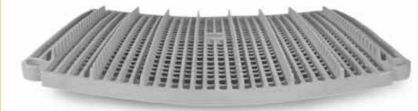
Deformation after 9 month
